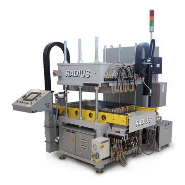
A 130 Ton RTM & SQRTM press with both heating and cooling capability.
