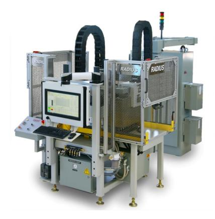
An 800° high temperature press with both heating and cooling capability.
